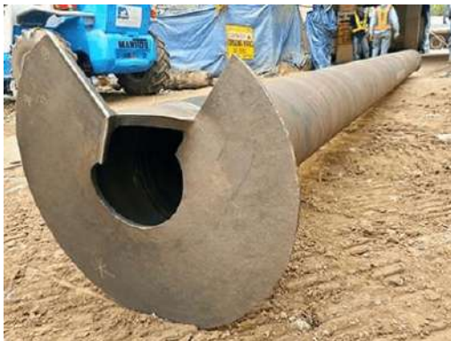
Figure 1. Continuous spiral helical pile
