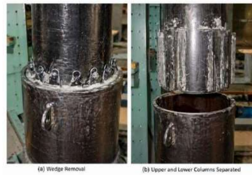
Figure 5. Connection disassembly procedure
